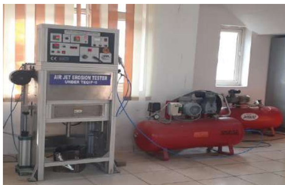
Fig. 1. Macrograph of the air jet erosion test rig used for high-temperature erosion testing
