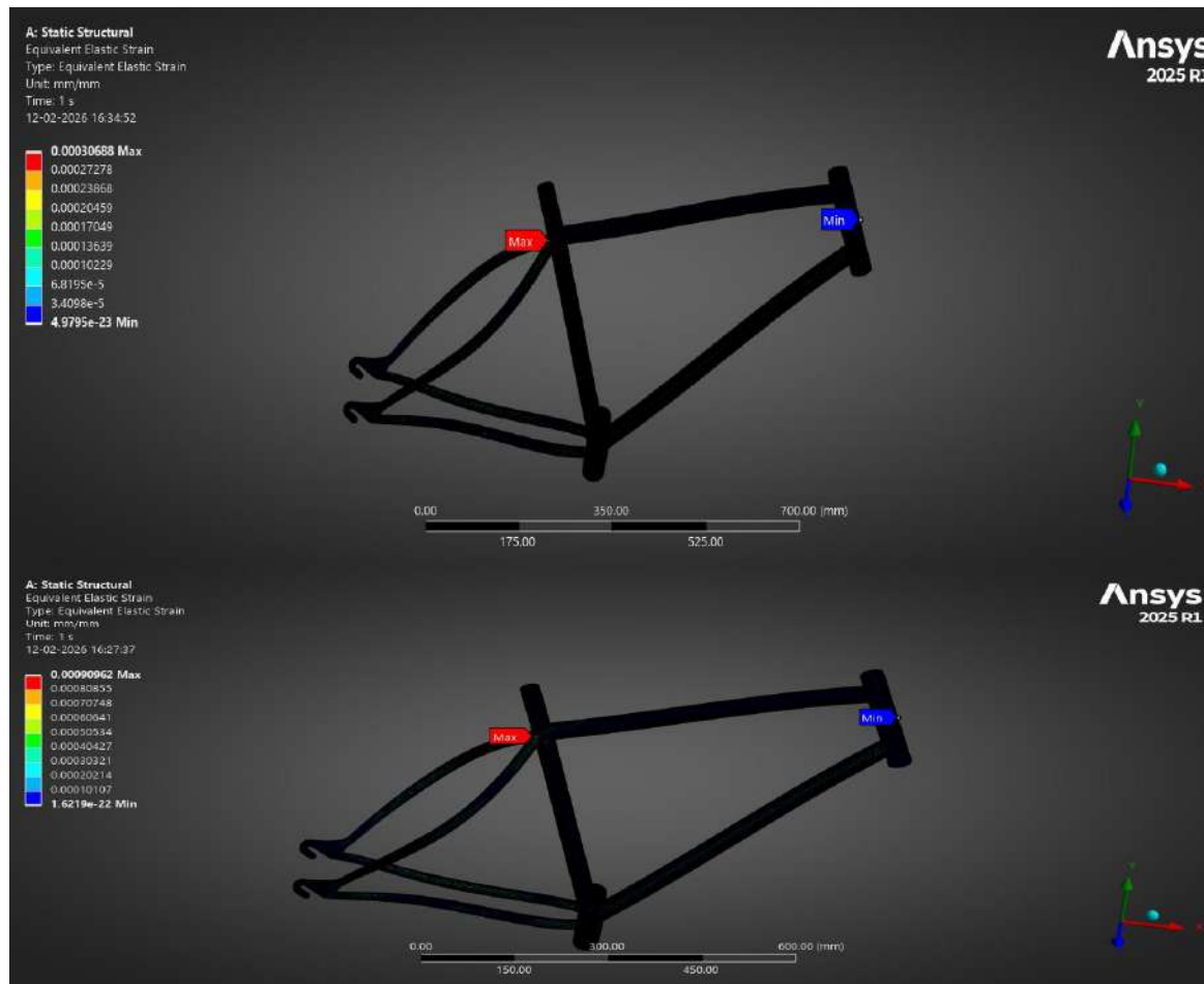
(i) Steel AISI 4130(ii)Aluminium 6061-T6
