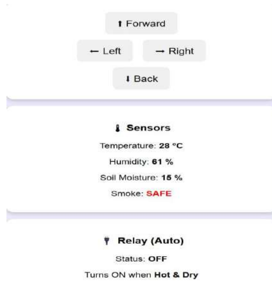
Fig. 2: Web-based IoT ( Internet of Things) dashboard for real-time agriculture robot control and monitoring
