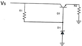
Given that the Zener diode breakdown voltage is 5V, the source voltage is 15V, the output voltage is 10V, R4 =  $2k\Omega$ ,  $\beta$ =99, R1= $2k\Omega$ .
